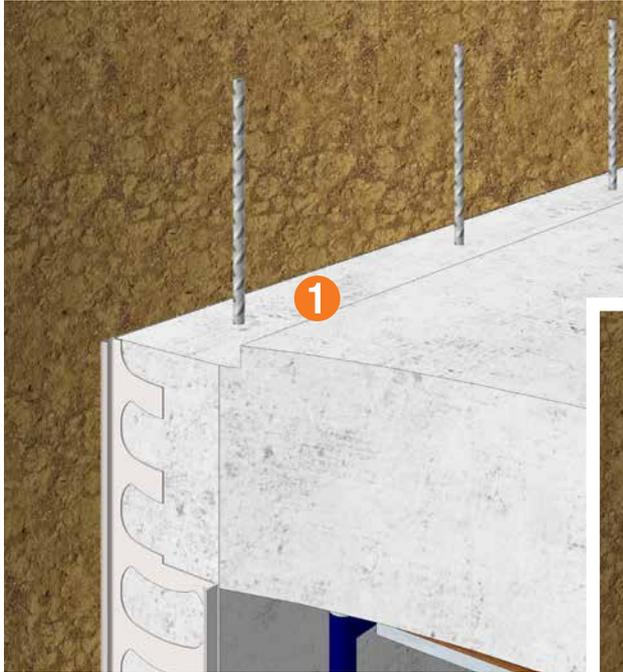
**1** Ensure that the suspended slab surface is free from debris and the level is checked and corrected as required. The Project Engineer should be consulted in relation to correct starter bar placement.
