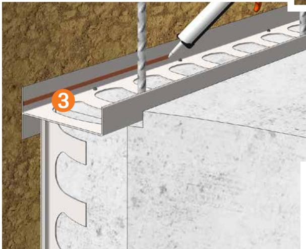
**3** Rediwall® J Track is then placed in the required location and fixed to the concrete slab using a masonry fixing gun or drill and anchor masonry fixing system. Fix with fasteners each side of the track at 500mm centres for walls up to 5m height, or at 250mm maximum centres for walls over 5m height.
