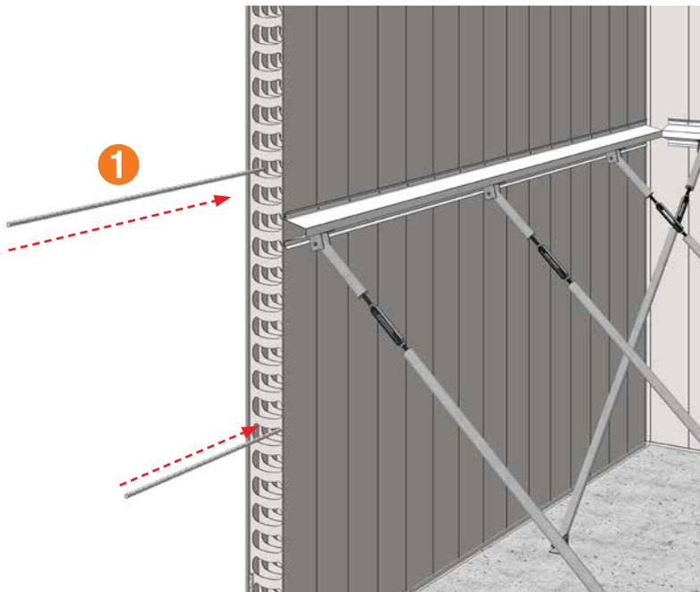
**1** Horizontal reinforcement bars should be placed into the wall when it reaches a suitable length. Generally the wall is slightly longer than the steel bar length. Slide the reinforcement bar through the rediwall® profile ensuring that the bar will maintain the correct overlap with the previous and subsequent bars where applicable.
