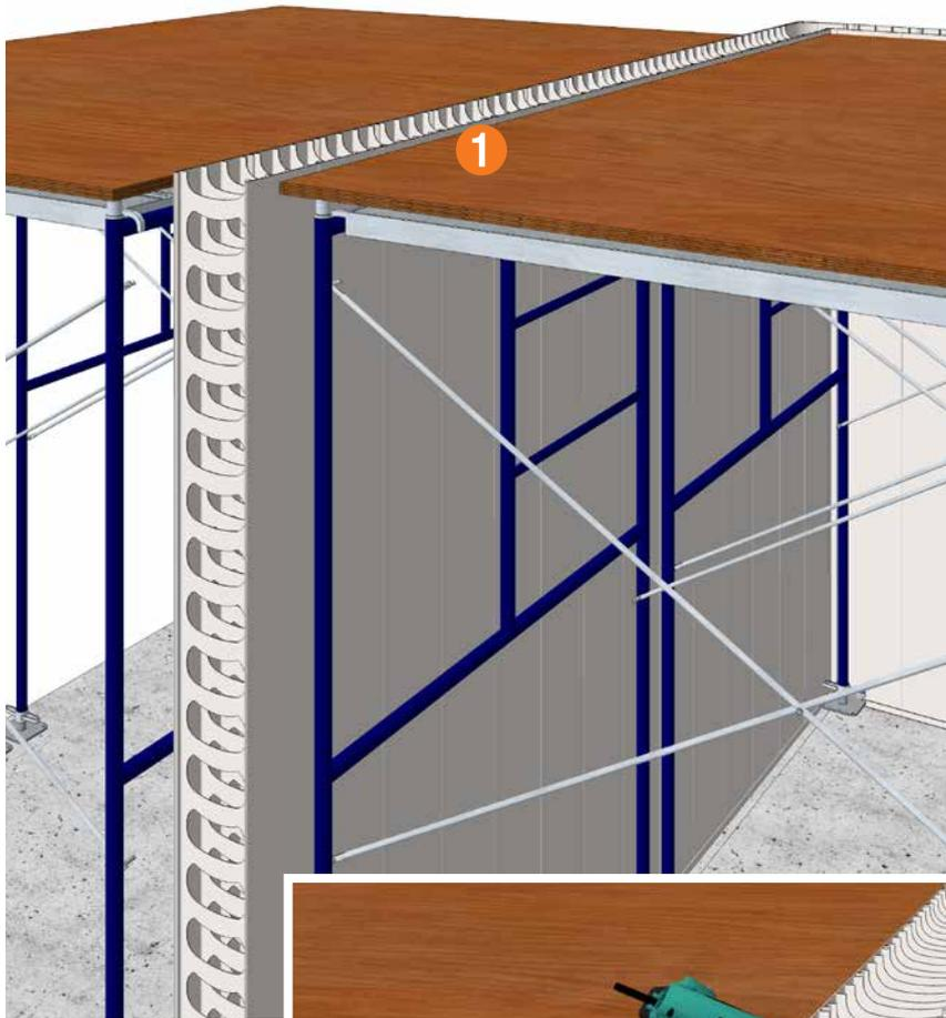
Rediwall® systems 3.3m or less in height that are being installed in conjunction with a formwork deck can be braced by being fixed directly into the form ply deck.
