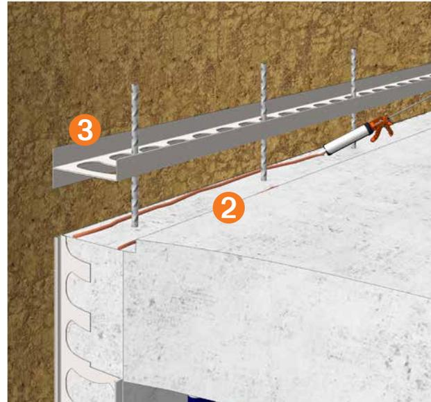
**2** Two beads of polyurethane sealant or as per waterproofer's details, must be applied in accordance with the manufacturer's instructions under the rediwall® floor track (one on each side of the track) on all external walls.
