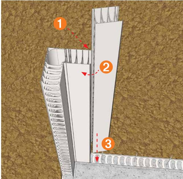
**1** From your chosen starting location, hook one side of the rediwall® panel together making sure that the panel is above the slab starter bars.
