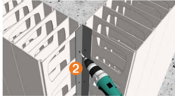
**3** Install the three corner angle brackets at the top, middle and bottom of the panels avoiding the location where final wall bracing will be fixed to the walls.
