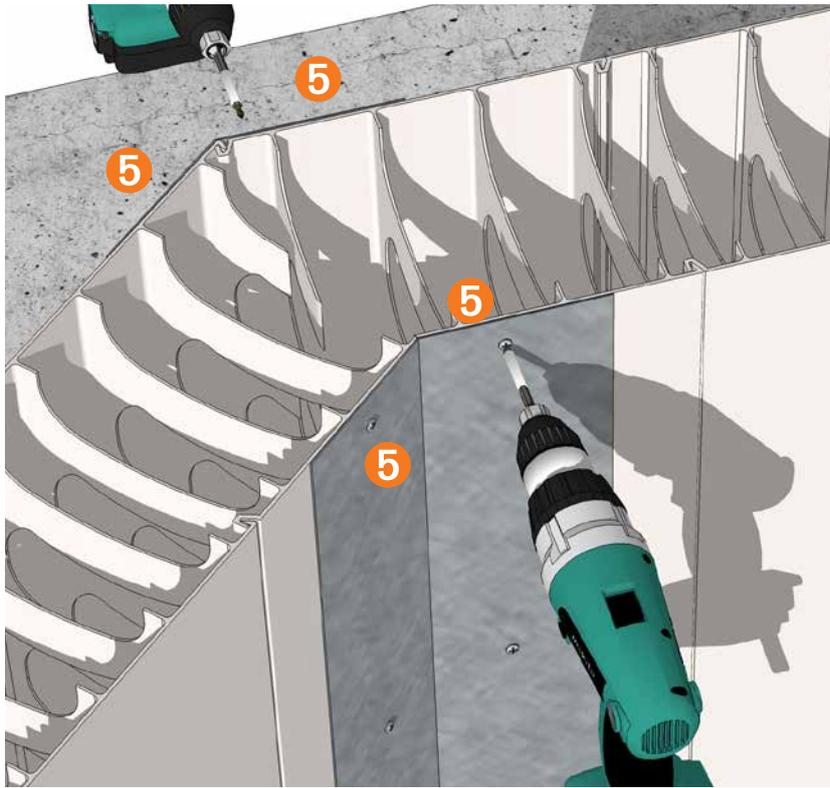
**5** Screw fix appropriate colorbond steel angle squints at maximum 150mm centres to both sides of the internal and external corner junctions.
