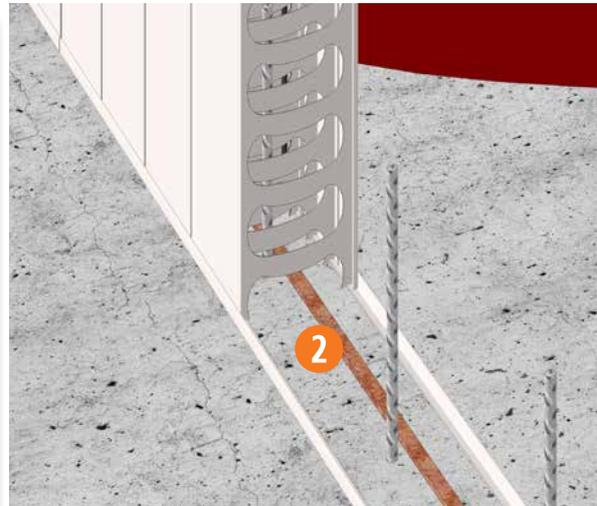
**3** Install the remaining rediwall® panels as per the standard installation method. Complete the tank with the required steel reinforcing as per Engineer's details.
