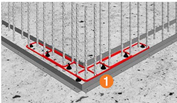
**2** Assemble the corner with 2-3 panels (or enough to fully accept the ligatures) for each leg of the corner and screw fix together at the joints. Install internal corner angle (standard 30x30mm angle) to one of the corner lags - fixing to the male end of the panel using tek-screws (type-17 metal) Panels should be ideally be laid down.
