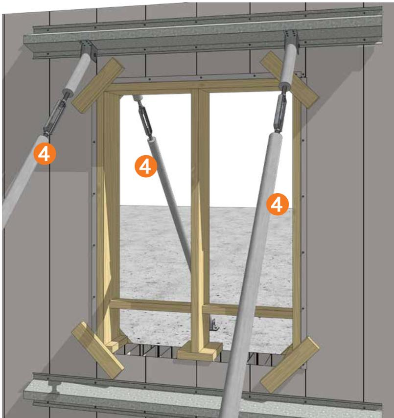
**4** The whaling plate is connected to angled braces (at 1100mm maximum horizontal spacings) anchored to deadmen or the floor slab, in order to hold the opening plumb.
