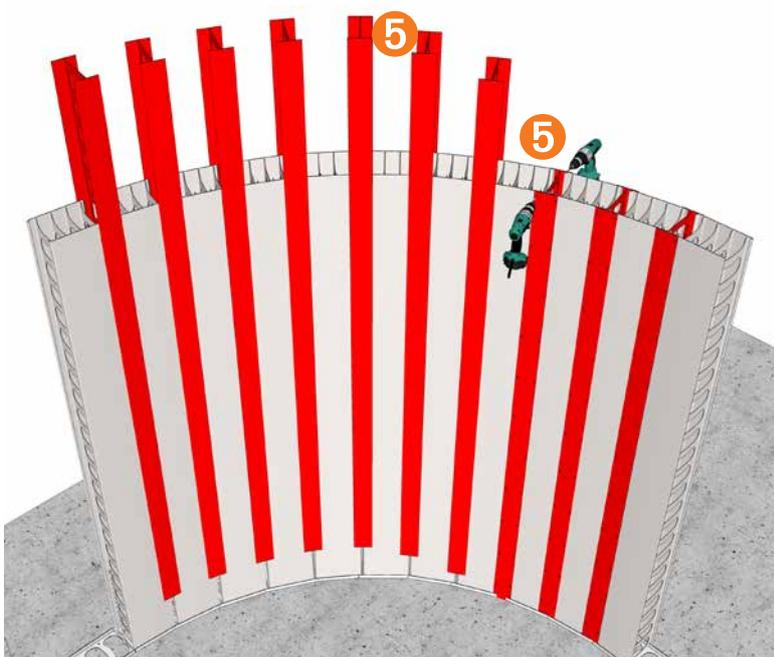
After installing the curved floor track, continue the wall by erecting panels in place allowing a small direction change in each wall segment. Screw fix panels to the floor track as erection proceeds.
