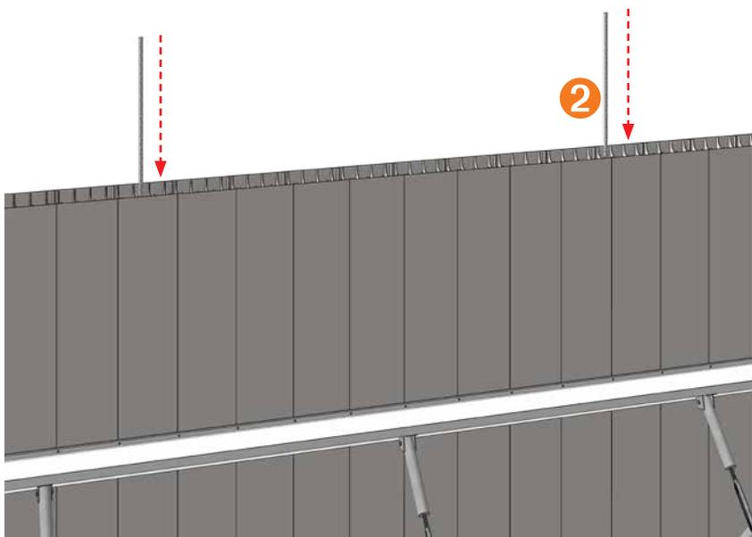
**2** Vertical reinforcement bar should be placed vertically into the rediwall® profile, weaving between alternate horizontal bars. Ensure that the bar will maintain the correct overlap with the previous and subsequent bars where applicable.
