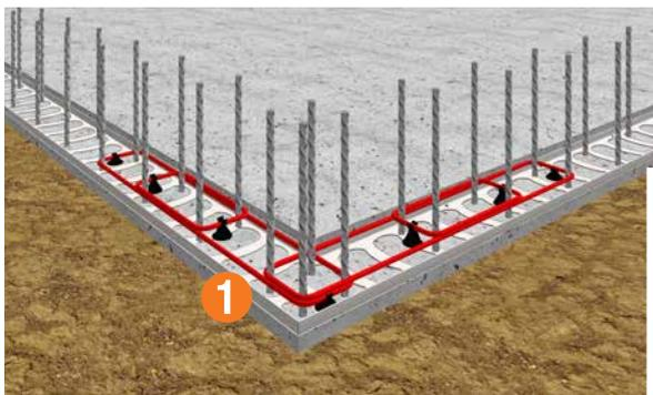
**3** Install the ligatures up to the level of the starter bars into the corner assembly. Locating as close as possible to their final position.
