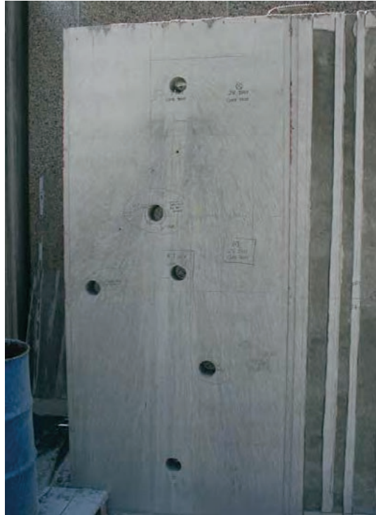
CORE DRILL TEST PANEL
