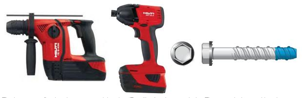
The braces are fixed to the concrete slab using 'Excalibur' style screw bolts. The screw bolts are driven into a hole that has been pre-drilled (using cordless rotary drill with appropriate sized masonry bit) using cordless impact wrench with appropriate sized impact socket.
