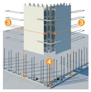
Install upper corner panels on top of lower corner panels. The panels can be installed manually or using crane depending on the panels size. Fix internal corner angle to the first upper panel to be installed as per step 2. Then plumb and brace lower panel 1 and upper panel 1 as per the standard procedure.
